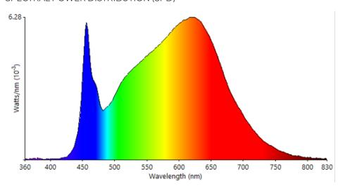
Testing was performed in accordance with LM-79-08.
